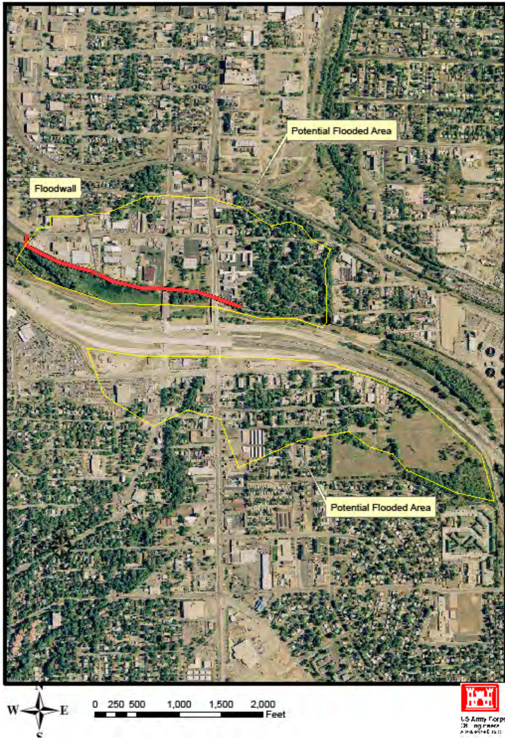
Figure 4-6. Flooding at Tejon and Nevada Bridges.
