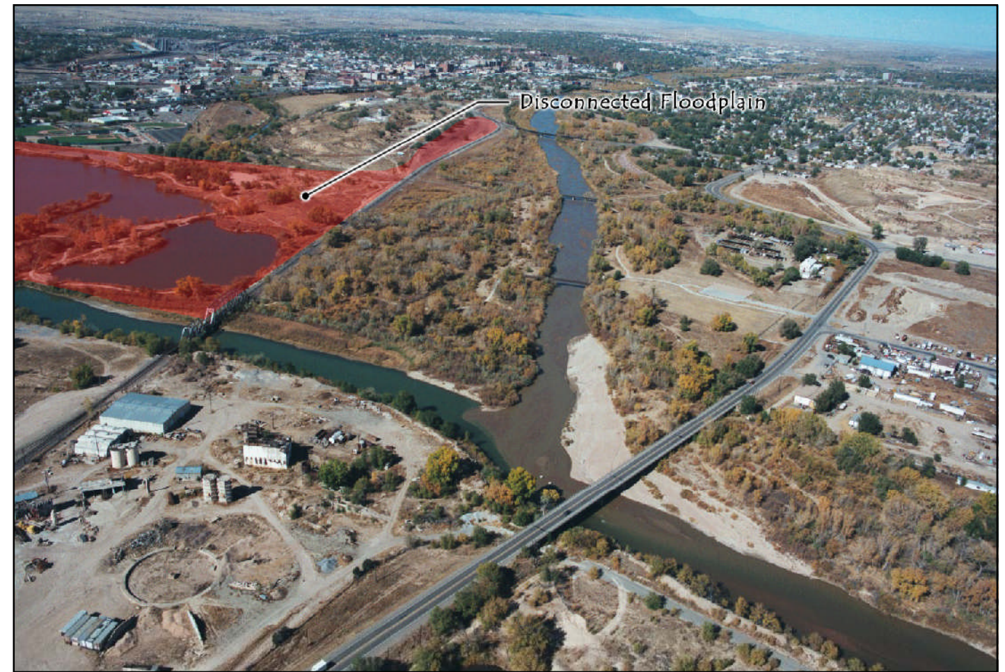
Figure 1.11 - Avoid Encroachment of Parallel Boundaries that Disconnect Fountain Creek from its Floodplain
